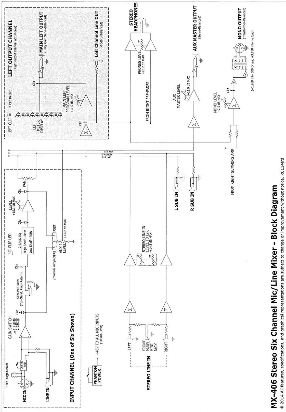
MX-406 Stereo Six Channel Mic/Line Mixer - Block Diagram
