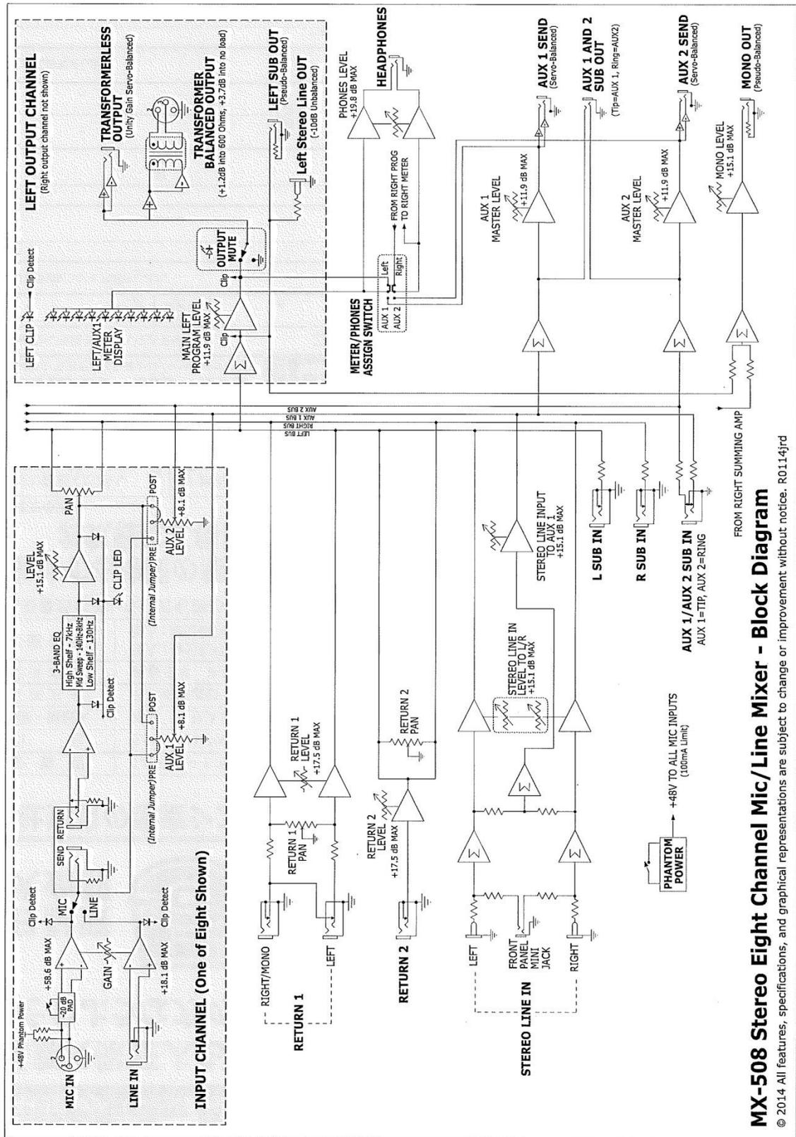
**MX-508 Stereo Eight Channel Mic/Line Mixer - Block Diagram**
